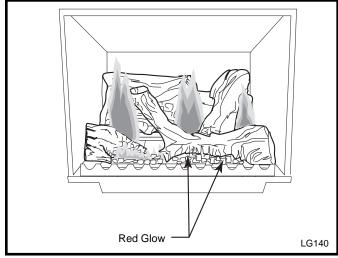
**Fig. 68** Correct flame pattern.
